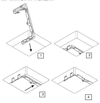
The claws of the support are positioned against the desk. If the cutout is not properly done, screw the support in the corners
