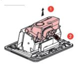
b) Insert the cable (flexible cable only) until the end stop (figure 3) then screw the cable clamp back (figure 4)  $\,$
