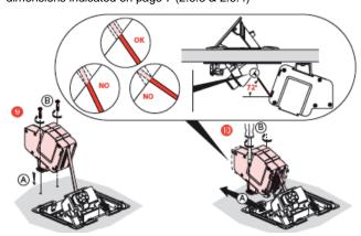
Adjust the retractor support (pop up open) so that the cable makes a straight line (avoid any contact with the edge of the cover)
