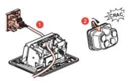
d) Put the cable in its receptacle and put the cable exit back
