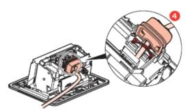
f) Put back the top part of the insulation casing and screw to end the installation
