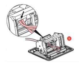
Connect the socket and clip it on the frame
