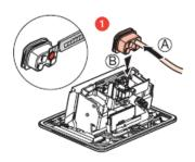
d)- Pass the cable through the frame to connect the sockets
