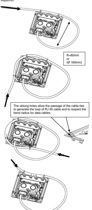
Note: if installation with several cables, they must be attached together using a cable tie
