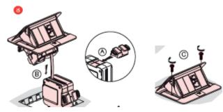
Fix the support of retractor under the desk according to the dimensions indicated on page 7 (2.6.3 & 2.6.4)
