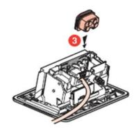
e) Lock the cable using the supplied cable tie
