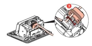
f) Put the insulation casing back
