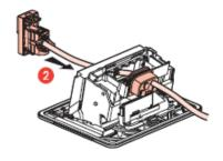
e) Put the cable exit back and lock the cable using the supplied cable tie
